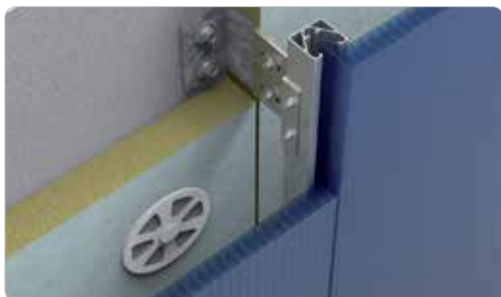
JUNCTION OF ADJACENT PANELS Paneling fixes(connects) to the masonry wall and secures to fit insulation material and allow air-circulation
